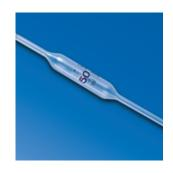
**Full pipettes (PP)** Highly transparent, break resistant. In six sizes from 1 to 50 ml.
