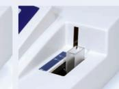
Round tubes (16 mm OD) and rectangular cuvettes (10, 20, 50 mm) can be used without any adaptor.
